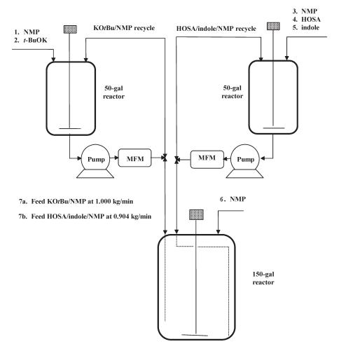
Figure 1. Process flow scheme.
