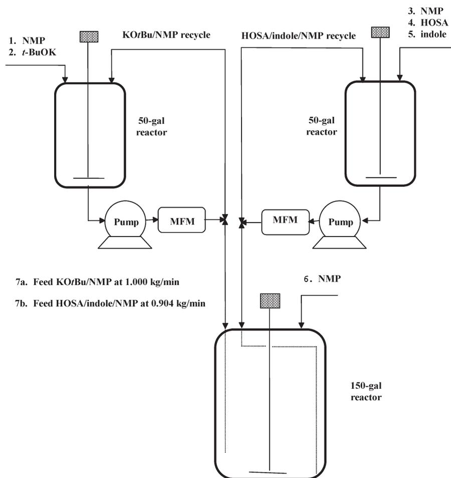
Figure 1. Process flow scheme.
